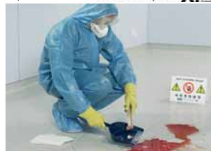
Figure 2: Removal of liquid contamination using the BERNER SpillKit XP
