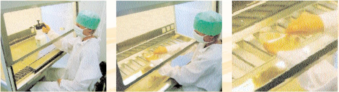
Fig. 4: Testing for the Cleaning Index of the working space, working surface and collecting basin in accordance with EN 12469
