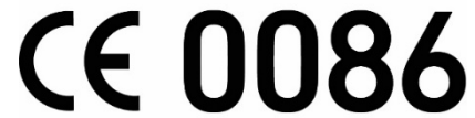
Figure 6: Example of CE mark with the four-digit identification number of the notified body
