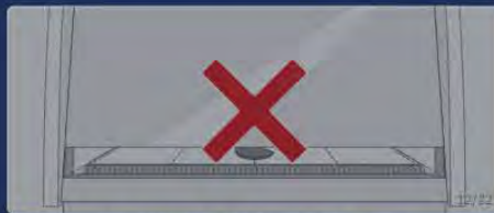
No strong heat sources (e.g. gas burners) in the workspace!
