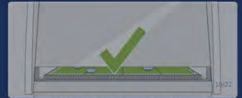
Safe area: Closed work surface!
